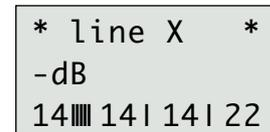
inputs: set 'Line Links' to 1>2.3. Slaved line faders (I) have no balancing activity, they get their gain value from the master (||||).
