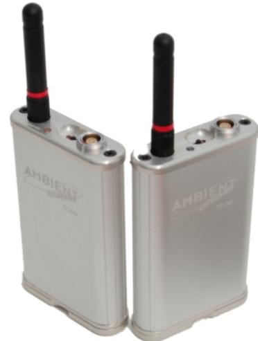
The units are powered by two AA batteries and use about 7 mA in RX mode, 12 mA when in TX.
