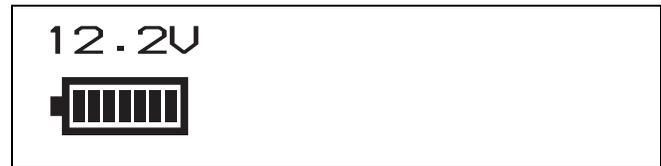
As the battery pack discharges, the segments go out from left to right. When the battery pack is almost exhausted (NEAR END), the voltage indication and the tally indicator start to flash, and an intermittent warning tone sounds in the headphones. When the battery pack is completely exhausted (END), the corresponding warning indication lights, the tally indicator starts to flash at a higher rate, and the headphones warning tone sounds continuously.
