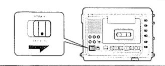
2 Press the STOP button if the tape transport is operating.
