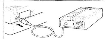
3 Connect the AC adaptor to a wall outlet using the power cord supplied.
