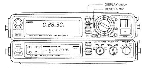
While the tape transport is operating, the time display shows the tape position.
