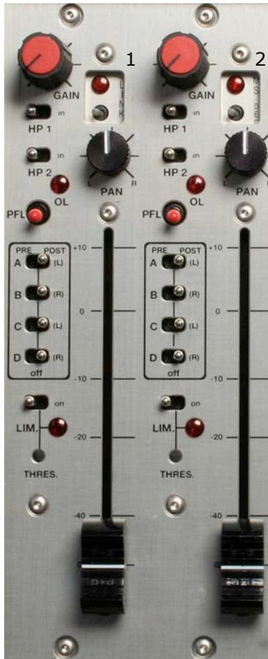
Any pair of mono channels can be converted to stereo pairs.\* The cosmetic difference is that the Pan out switches are replaced with Link & MS Decode switches with LEDs above.
