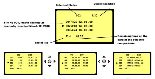
The display shows the length, the date of recording, the time at the record start and the type of file format.
