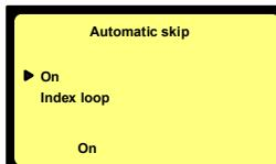
When "Index loop" is chosen, only the selected index will be played back in loop mode. To select another index use the skip keys (3) & (6). To playback the same file, press the "REWIND" key (3) shortly and push play again.
