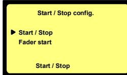
When "Record/Stop" is selected, the machine starts recording at a momentarily short-circuit on the "Start /Stop" input, and stops recording on the next short-circuit.
