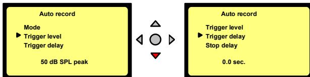
The "AUTO RECORD" menu permits to turn on or off the auto record mode. This mode of recording permits to start a recording automatically depending on the settings of the different parameters described below. Once the parameters set, put the machine in the record mode. The recording will start once the requested level and length of any incoming sound is obtained.
