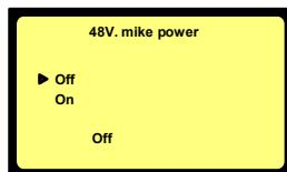
If Phantom microphones are used the 48V must be turned on. This selection needs to be confirmed by pressing the right arrow key. On the main display, the text will appear next to the battery status.
