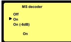
The "ON (- 6 dB)" is to reduce the saturating danger in case that the recording is made with high input levels.
