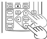
To return to normal playback, press the ► button or the VAR.SEARCH button on the remote control.
