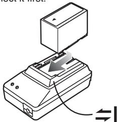
**2** Plug the AC cord into the power outlet.
