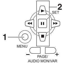
**To select thumbnails:** Select the thumbnails (the yellow frame moves) using the  $\triangleleft$  and  $\triangleright$  buttons, and press the  $\square$  button (the color of the frame changes to blue-green). Press the  $\square$  button again to deselect the clip. To scroll the pages, press the PAGE (- or +) button.
