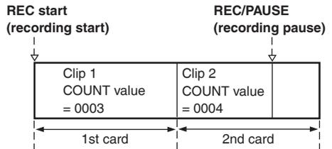
If the clip thumbnails are displayed as shown in the example above or their properties are indicated using a P2 device, the thumbnail and COUNT value of clip 1 will be displayed.
