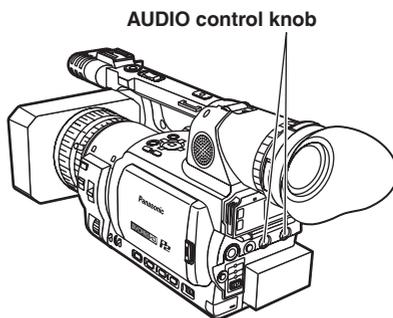
Use the AUDIO control knob to adjust the recording level of the built-in microphone or of audio signals input through the INPUT 1/2 (XLR 3-pin) terminal.
