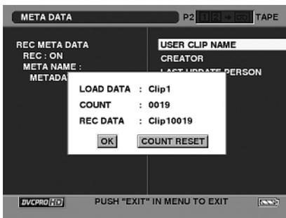
When a P2 card with a memory capacity of 8 GB or more is used in this unit and a one-time continuous recording exceeds the prescribed duration (approx. 5 minutes for DVCPRO HD, approx. 10 minutes for DVCPRO50 or approx. 20 minutes for DVCPRO or DV) or when a one-time recording extends over more than one P2 card, the recording concerned will automatically be undertaken as a separate clip.
