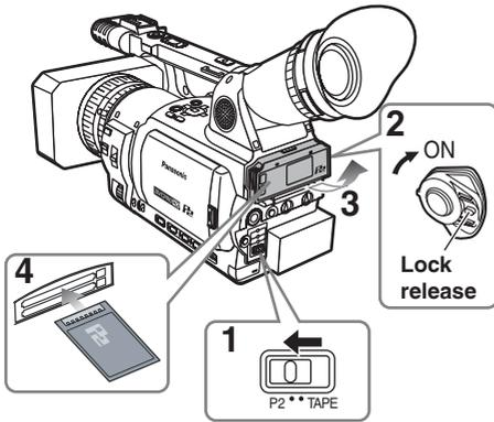
Do not operate the MEDIA switch when the power is switched ON.
