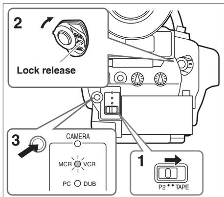
**1** Before turning the POWER switch to ON
