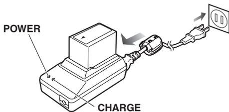
**3** When the battery is charged, the CHARGE lamp on the AC adapter goes out.
