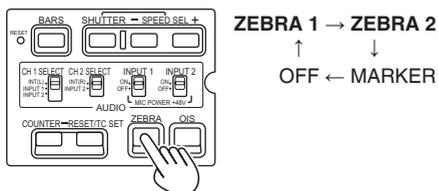
In the setup menus, DISPLAY SETUP screen, ZEBRA DETECT 1 and ZEBRA DETECT 2, set the brightness for the zebra patterns. (Page 113)
