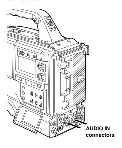
2 Set the AUDIO IN switch or switches for the channel or channels to which the microphone or microphones have been connected to "REAR."
