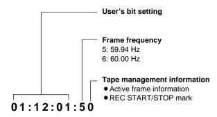
When the camera's video signals are being recorded
