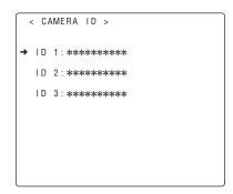
**3** When the JOG dial button is pressed, the arrow (cursor) moves to the ID input area, and the input mode is established.
