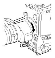
4 Push the cable into the cable clamp, and connect it to the LENS socket.
