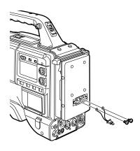
**3** Connect these connectors with the connector on the AU-MA402H battery case.
