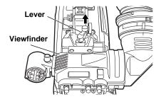
2 Loosen the lever for securing the viewfinder in the back/front and sideways directions.
