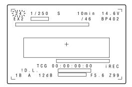
${f 3}$  Press the synchro scan adjustment switches ("+" and "-") to set the desired frame rate.
