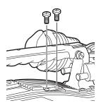
2 Attach the mic holder to the main unit using the screws provided with the AJ-MH700P mic holder.
