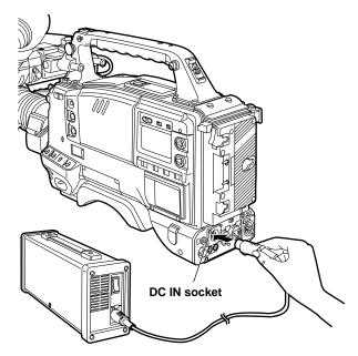
2 Set the power of the AC adapter to ON.
