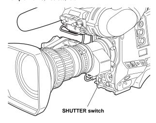
3 Press the SHUTTER switch to the SEL position again, and repeat this until the desired mode or speed is displayed.
