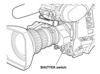
2 In the SYNCHRO SCAN mode, continuous switching inside the 3.0 deg to 350.0 deg (0.8% to 97.2%) range can be achieved by pressing the SYNCHRO ("+" and "-") buttons.
