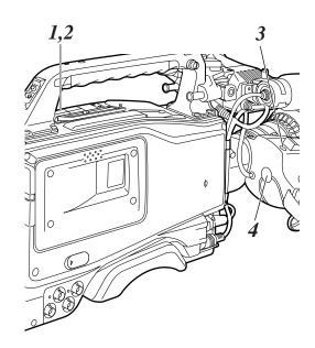
The functions of a VTR START/STOP button can be assigned to the USER1 or USER2 button on the unit's side panel on the CAM SW MODE screen of FILM (CAM) MAIN MENU 2, and this button can then be used to perform the start and stop operations.
