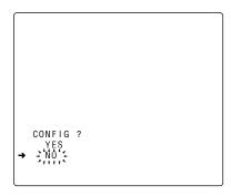
To proceed with the formatting of the setup card, turn the JOG dial button to move the arrow (cursor) to YES, and press the JOG dial button. When the formatting of the card is completed, the following message appears.
