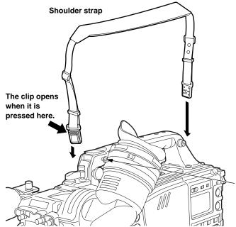
To detach the shoulder strap, open the clips on the mounting parts and detach.
