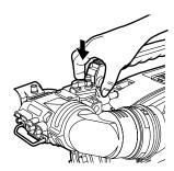
4 Tighten the stopper screw firmly.
