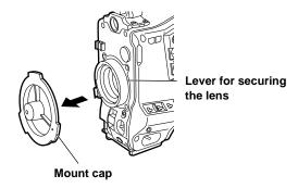
2 Align the center mark of the lens with the groove in the top center of the lens mount, and attach the lens.
