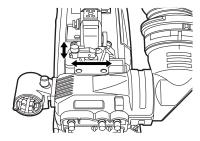
**4** Tighten the lever for securing the viewfinder in the back/front and sideways directions until it locks the viewfinder in place.
