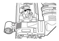
**3** Move the viewfinder in the back/front and sideways directions, and adjust its position.
