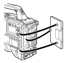
2 Attach the connectors provided with the NP/BP adapter plate to the positions shown in the figure.
