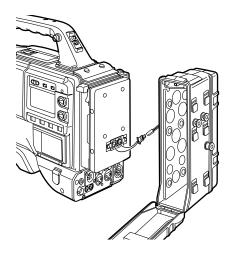
4 Attach the AU-M402H battery case.
