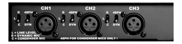
Input Level Switch: Line Level (0dB Gain), Dynamic Mic (60dB Gain), Condenser Mic (45dB Gain)
