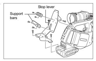
When using the optional CH-910, hook it onto the support bars and secure it with the stop lever. To detach the CH-910, press the stop lever in the direction of the arrow and pull it off the support bars.
