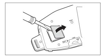
2. Using a pair of cutters or tin snips, cut the 4 indicated plastic joints and remove the cover.
