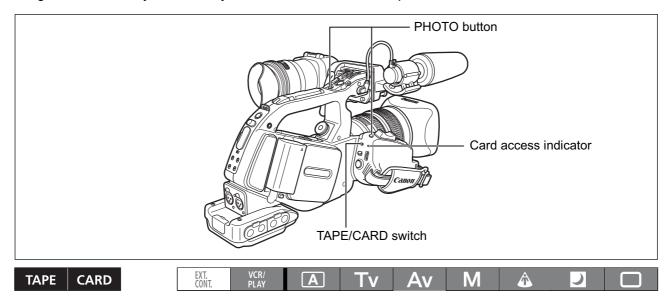
1. Turn the POWER dial to a recording program and move the TAPE/CARD switch to ....
