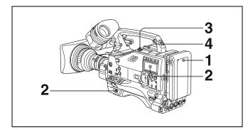
Attach a fully charged battery pack.
