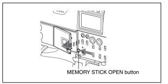
**2** Hold the "Memory Stick" with the notch facing downward and the label side facing toward you, and insert the "Memory Stick" into the "Memory Stick" insertion slot until it clicks into place. Then close the cover.
