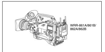
**3** Connect the tuner power cord to the DC OUT connector of the camcorder, and the audio output cable to the AUDIO IN CH1 or CH2 connector.
