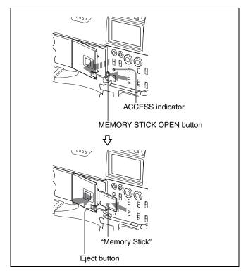
Open the cover of the "Memory Stick" compartment by pressing the MEMORY STICK OPEN button and insert the "Memory Stick."
