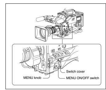
**1** Open the switch cover first. Set the MENU ON/OFF switch to ON while pushing the MENU knob.
