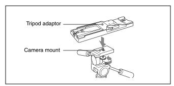
**2** Mount the camcorder on the tripod adaptor.
