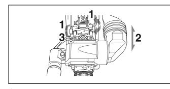
1 Loosen the viewfinder front-rear positioning lever and the LOCK knob.
