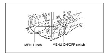
1 Set the MENU ON/OFF switch to ON while holding down the MENU knob.
