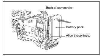
**2** Slide the battery pack down until its "LOCK" arrow points at the matching line on the camcorder.
