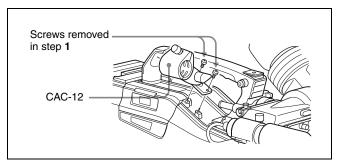
**3** Open the CAC-12 and remove the microphone adaptor.
