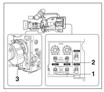
**1 To record stereo sound:** Set both AUDIO IN CH-1 and CH-2 switches to FRONT.
