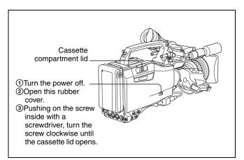
You need not return the screw to its original position after taking out the cassette. Although the cassette compartment lid is not locked, turning on the power makes the cassette lid operable again.
