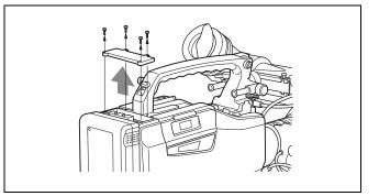
**2** Insert the WRR-855A/855B, and fasten the four fixing screws.
