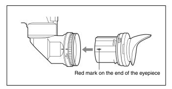
**3** Turn the eyepiece locking ring clockwise until its "LOCK" arrow points at the red mark on the viewfinder barrel.
