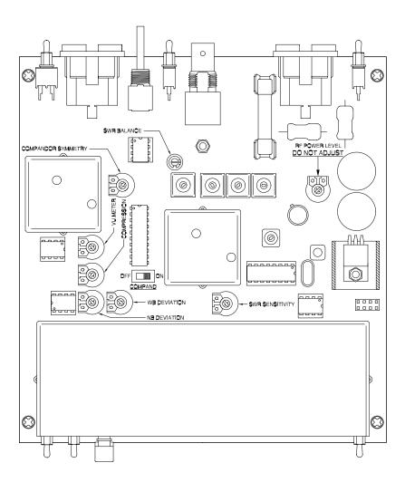
**NOTE:** The <u>Compand Switch</u> must be set to the "**ON**" position for automatic companded and non-companded operation with channel selection. The "**OFF**" position is only used for testing.
